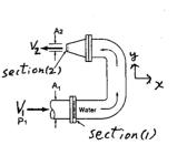
At section 2: the pressure is atmosphere; the velocity is  $V_2$ ; the area is  $A_2$
