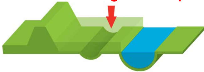
Lowering of floodplains
